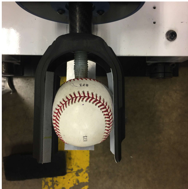
Fig. 2.8: MLB baseball in the flex tip in the Top Loop orientation as viewed from the top. Seam effects for this orientation cause advanced separation on the top of the ball resulting in a downward force.
