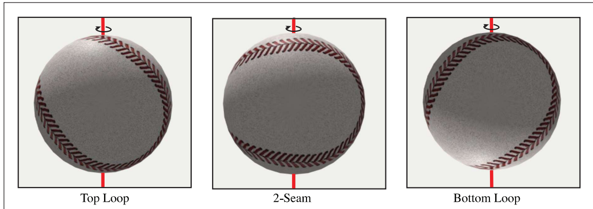
Fig. 2.3: The three seam orientations used in this study. The “Top Loop” orientation has a seam that is always near the top spin pole. The “Bottom Loop” has a seam that is always near the bottom spin pole. The 2 seam has no seam is near a spin pole. The Top Loop orientation is so named because a pitched spinning ball will appear to have a red loop spinning about the top pole. Similarly, the Bottom Loop appears to have a red loop spinning about the bottom pole.
