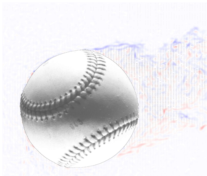
Fig. 1.2: A PIV image of an MLB baseball moving left at 90 mph with an imbalanced wake. The separation on the seam on the top of the ball is forward of the separation on the bottom of the ball causing an imbalanced pressure field on the ball. This ball will have additional down force due to the asymmetry of the wake.
