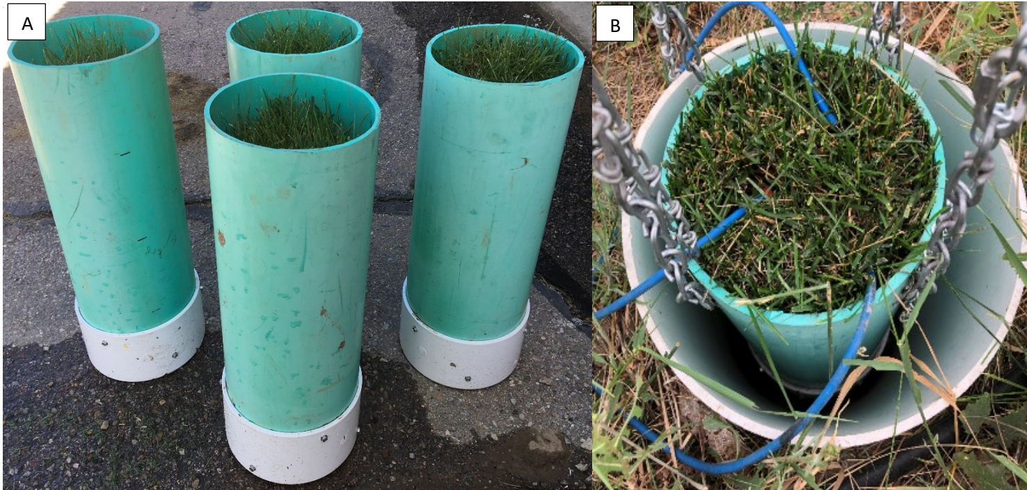
Fig. 2. (A) Four weighing lysimeters, constructed of PVC pipe, before installation at ground level. (B) A weighing lysimeter, hung by chains from a precision scale, installed at ground level with three drip irrigation emitters.
