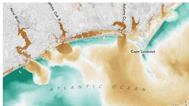
Figure 1: Combined VIS and IR data used to track debris after Hurricane Florence in 2018. Image by P. Fucile (WHOI)
