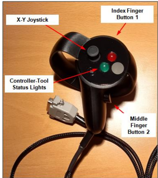
Figure 14: Left Hand Controller to Actuate Tools
