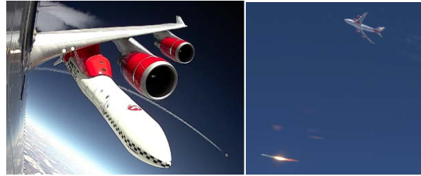
Figure 1: LauncherOne and Cosmic Girl, Virgin Orbit's small satellite launch platform.
