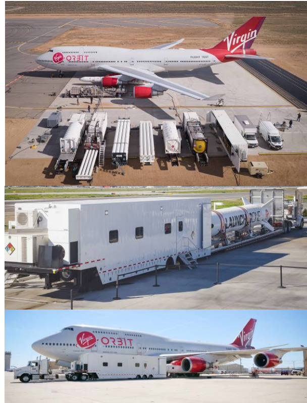
Figure 2: LauncherOne's rapid-response mobile ground support trailers are globally transportable.
