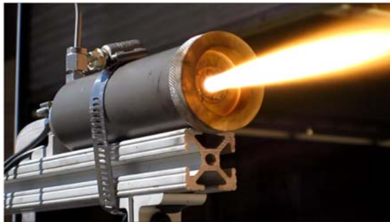
Figure 4: 25-N High Performance Green Hybrid Propulsion System During Test Firing Sequence. Credits: Utah State University
