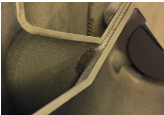
Figure 7: Example of Partial Fusion of Unsintered Powder
