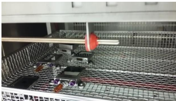
Figure 21: Sensors in thermal shock chamber
