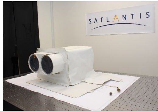
Figure 27: iSIM FM Thermal interface (beta cloth) fitting test.
