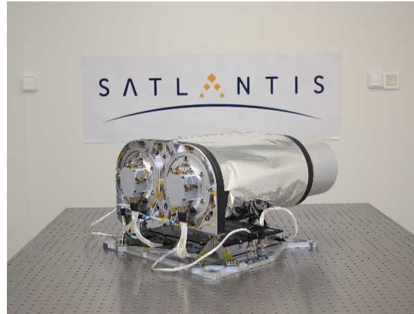
Figure 2: The Flight Model of the iSIM-170 payload. The electronic box is located directly below the opto-mechanical system (the base structure shown here is the mechanical interface plate with i-SEEP).
