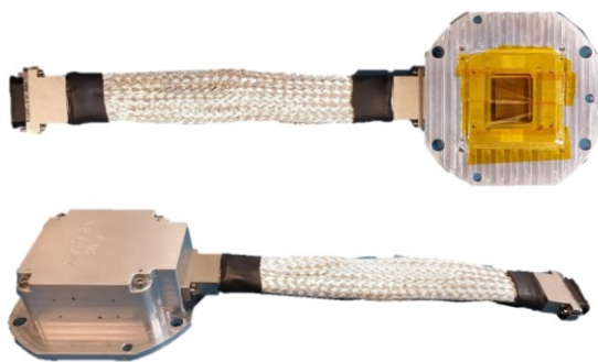
Figure 9: The Sentech COTS Camera assembled with the new case and interface.
