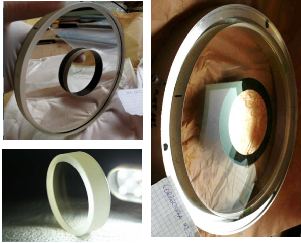
Figure 4: M1 (top left), FL (bottom left) and M2 (right) for iSIM-170. Note they are not to scale.
