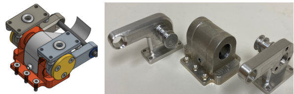
Figure 16. ATA 90 Degree rotary fluid joint: Nano90
