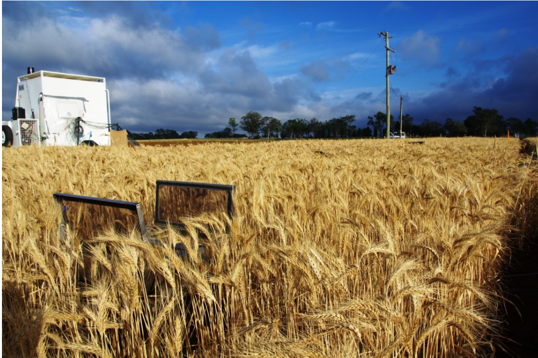
Figure 2-12 - Automated closed static chamber during the sampling campaign in wheat (see Chapter 3). The automated sampling unit and the analytical equipment are both housed in the white trailer seen in the background. Photo credit: Massimiliano De Antoni Migliorati.
