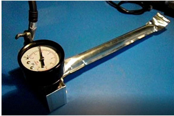
Figure 8: 4 atmosphere hold on RDR sample
