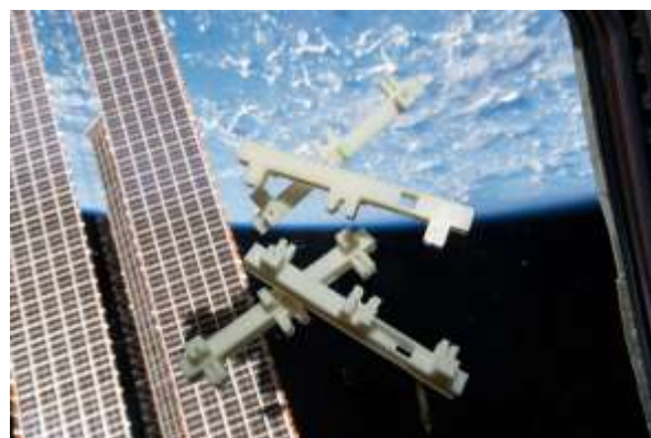
Figure 5: MakerSat-1 frame being 3D printed by the AMF printer from Made In Space aboard the ISS.
