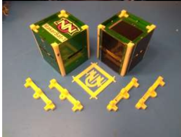
Figure 6: MakerSat-1 3D printed frame components aboard ISS
