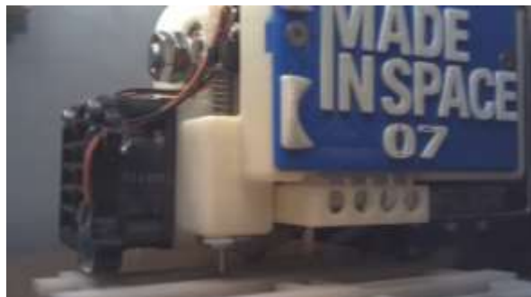
Figure 5: MakerSat-1 frame being 3D printed by the AMF printer from Made In Space aboard the ISS.
