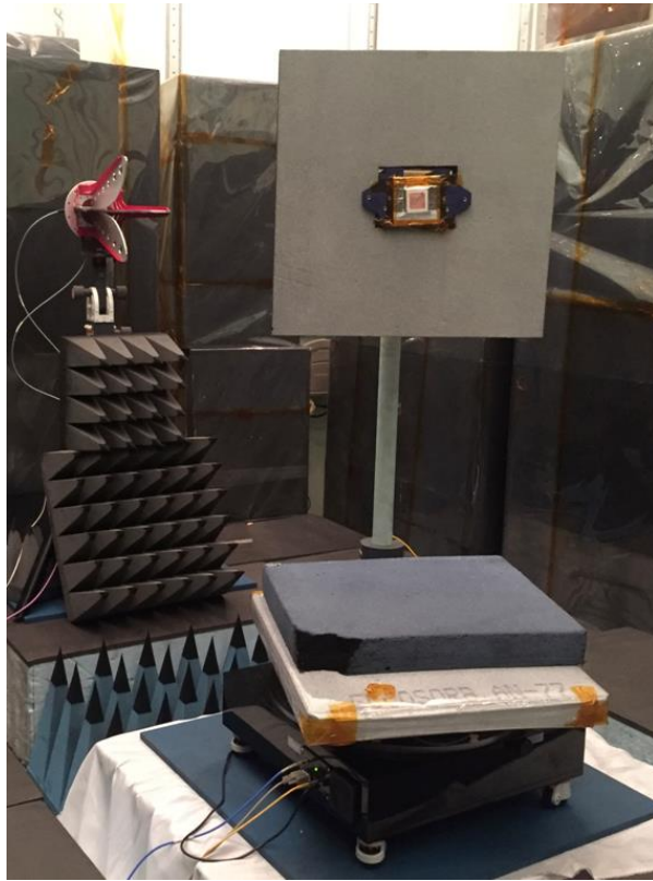
Figure 4.9: RHCP Patch in Antenna Testing Setup
