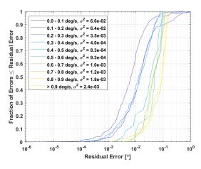
Figure 16: AC10-A Cumulative Distribution of Kalman Filter Residual Errors
