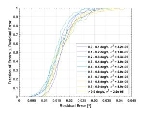
Figure 15: AC10-A Cumulative Distribution of Star Residual Errors
