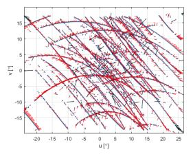
Figure 13: Star Matches Post-Distortion Correction. The blue dots are matched stars on the focal plane and the red lines represent the error.
