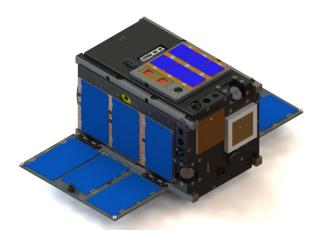
Figure 1: AeroCube-10 Spacecraft CAD Rendering
