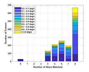
Figure 14: AC10-A Star Matches over a Range of Mission Slew Rates
