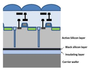
Figure 4: Schematic of the XQE-0920 Pixel Layout
