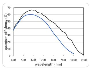
Figure 3: Quantum Efficiency of XQE-0920 (Black) vs sCMOS (Blue)
