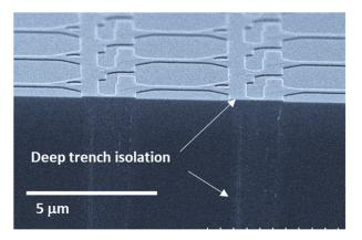
Figure 5: Scanning Electron Micrograph of the XQE-0920 Image Sensor
