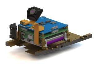
Figure 8: AeroCube-10 Star Trackers, Avionics and Harnessing
