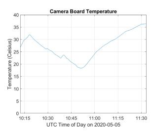
Figure 11: Camera Board PCB Temperature -AeroCube-10B, May 5, 2020
