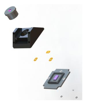
Figure 9: AeroCube-10 Star Tracker Sub-Assembly Exploded View
