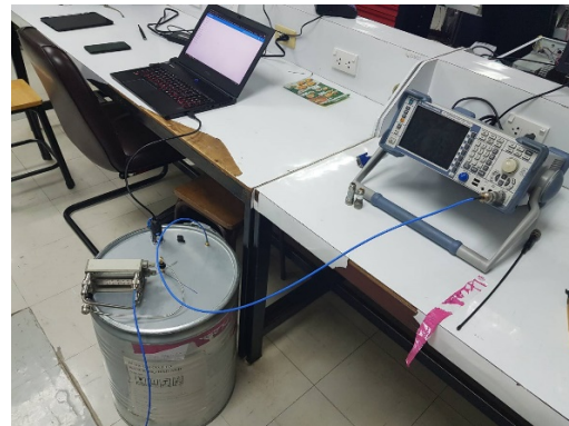
Figure 20: Spectrum analyzer set up to monitor the signal leakage
