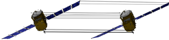
Figure 6: Example of feature vector matching on preliminary artificial data of a slightly rotated satellite. Model © NASA
