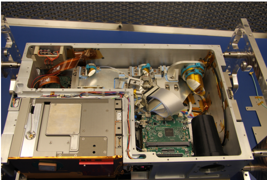
Figure 10: DeMi payload fully installed into spacecraft bus.
