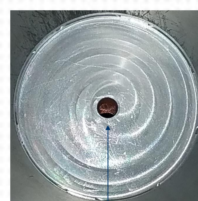
Misalignment of cryogenic shroud initially eclipsed apertures
