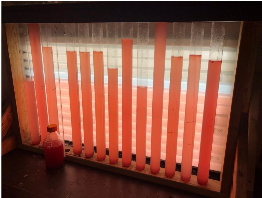
Figure 3. Growth of the PB23 strain just before the cell mass was harvested. Note that the differences in liquid height come from slight pressure differences between the connected tubes. This allowed more pressurized tubes to push liquid into less pressurized ones. One tube shattered under high pressure, and the culture was salvaged by growing it in a 1 L media bottle.
