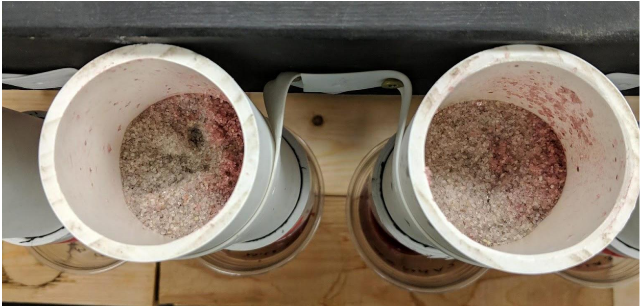
Figure 22. Sand after washing the cell biomass through the column. Compare to Figure 11 for an observation of the color difference before (Figure 11) and after (Figure 22).
