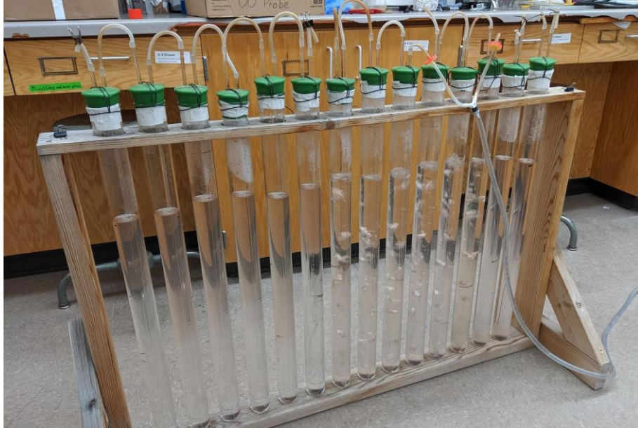
Figure 2. Bubbling nitrogen through the tubes to remove oxygen, and to mix the vitamins and inoculum thoroughly.
