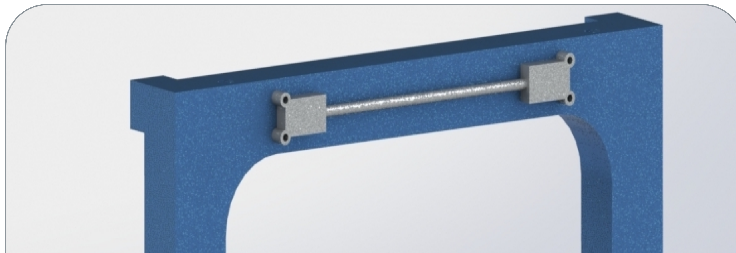
Preliminary mounting of hysteresis rods along the satellite's x axis. The hysteresis rod housing will be mounted to the bottom of the payload enclosure support tray.
