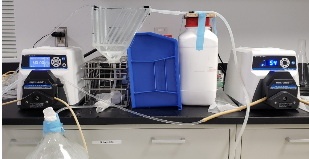
Figure 1. The set up for testing design prototypes is shown. This includes two separate inlet and outlet peristaltic pumps (left and right) sandwiching the initial lamella prototype.
