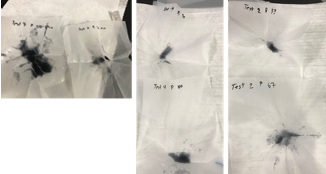
Figure 3. Dyed microcarriers separated from permeate and return streams caught on mesh from hydrocyclone tests. The microcarriers were weighted on the mesh to calculate the efficiency of separation.
