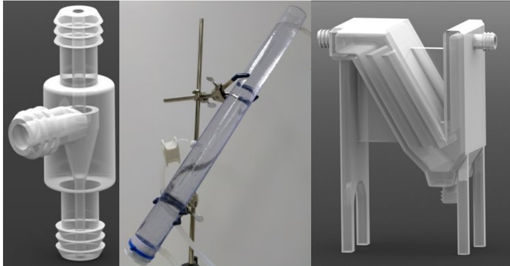
Figure 1. The redesigned SolidWorks model of the hydrocyclone separator, a picture of inclined settler, and the SolidWorks model of the redesigned lamella settling device. (left) Second hydrocyclone design modeled in SolidWorks. All dimensions taken from preliminary prototype were scaled down to millimeter scale, and inlets and outlets were modelled to have a diameter of \frac{1}{4} in. (center) Inclined settler prototype, pictured during settling experiment, the degree of incline controlled with test tube clamps and a stand. (right) Second lamella separator modelled in SolidWorks, modifications included a total volume reduction and inlet and outlet ports modified to a \frac{1}{4} in diameter.
