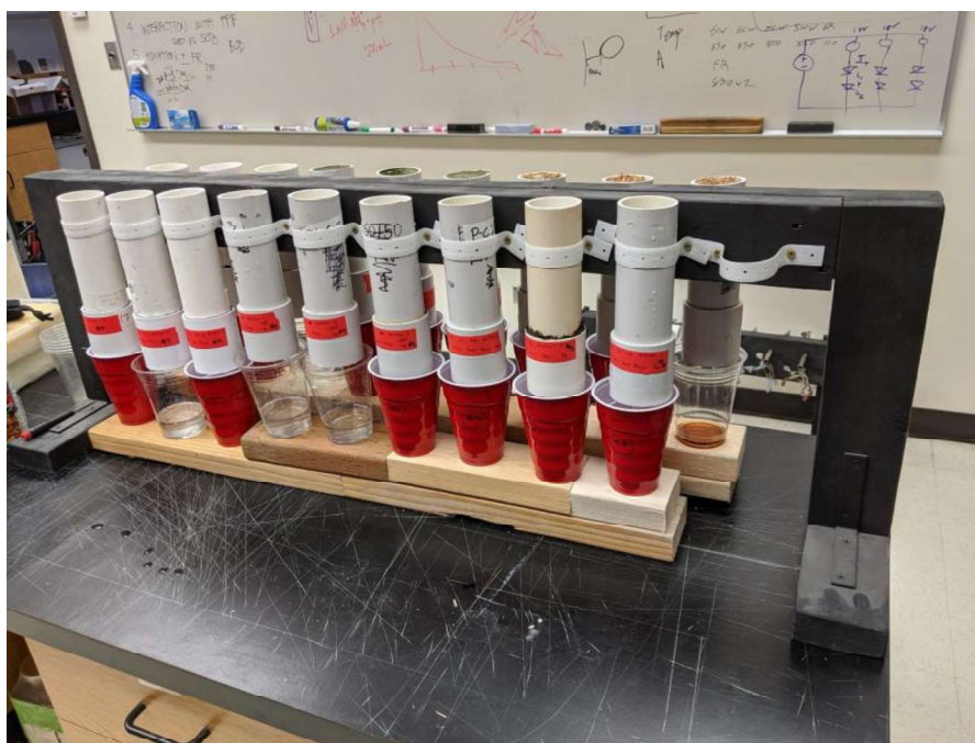
Figure 12. The columns used in the soluble nitrogen degradation study.
