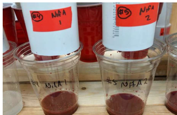
Figure 21. Cell biomass captured in leachate after flowing through the column. In previous experiments testing the system, the leachate was clear
