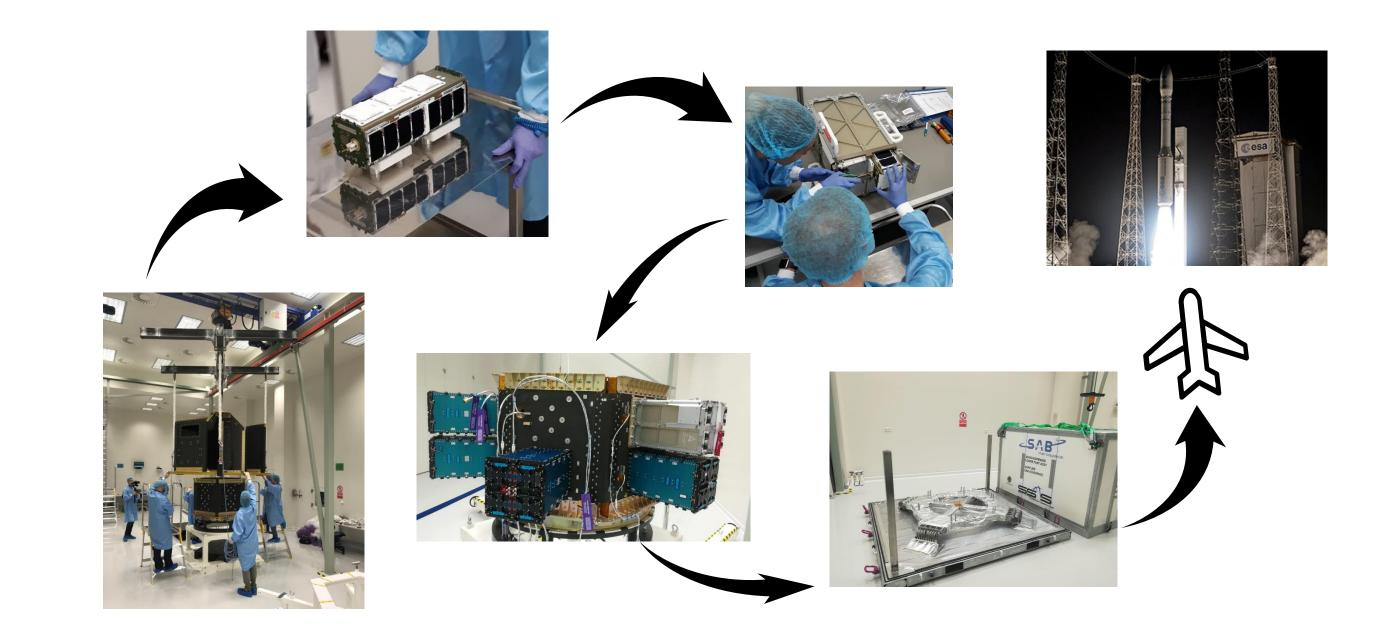
The SSMS Dispenser is the hardware developed to optimize multiple small satellite missions on VEGA and VEGA-C. The SSMS Dispenser is a modular structure which can be flexibly configured in order to be adapted to the specific satellite aggregate.
