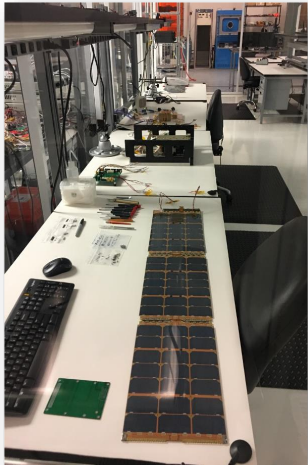
Figure 6. The Lunar IceCube spacecraft's solar array undergoing electromagnetic testing at Morehead State University.
