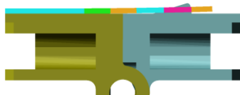
Figure 27: Latch Tab in Preloaded State when Hinge is Fully Deployed
