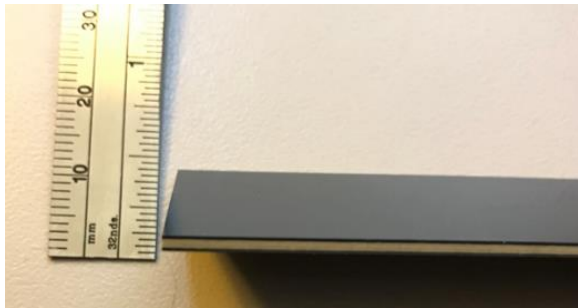
Figure 2: The CF-SF-CF Laminate is 0.060 in Thick
