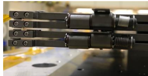
Figure 31: Hinged Edge Members Showing Rattle Gaps between Panels
