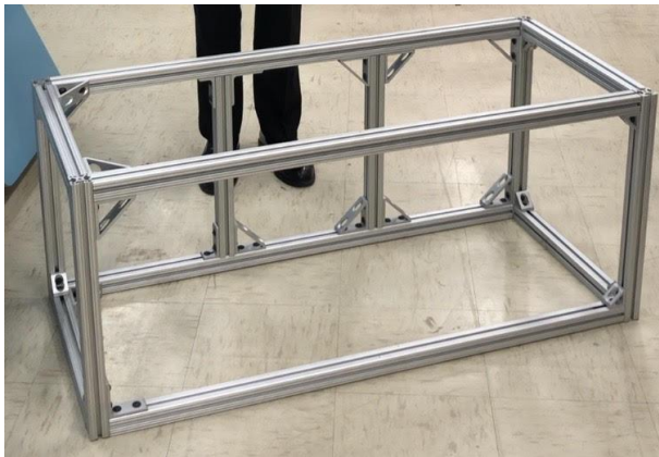
Figure 15: The first iteration of the CAGE made of 1.5" x 1.5" 80/20 aluminum beams
