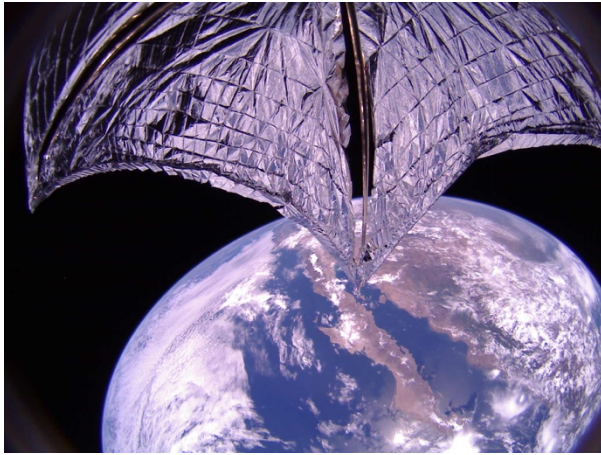
Figure 5: LightSail 2 sail deployment image, acquired shortly prior to reaching full deployment. Credit: The Planetary Society.
