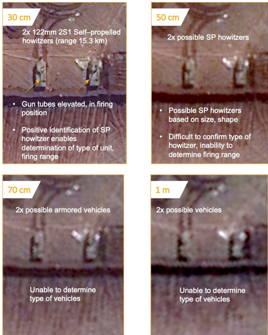
Figure 2. Only 30 cm resolution has sufficient detail to draw a meaningful conclusion about the type of military equipment in this image.
