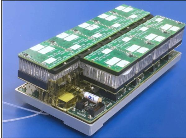
**Figure 5: Photo of 9-Microfluidic Cards with a Cal Cell and Manifold**
