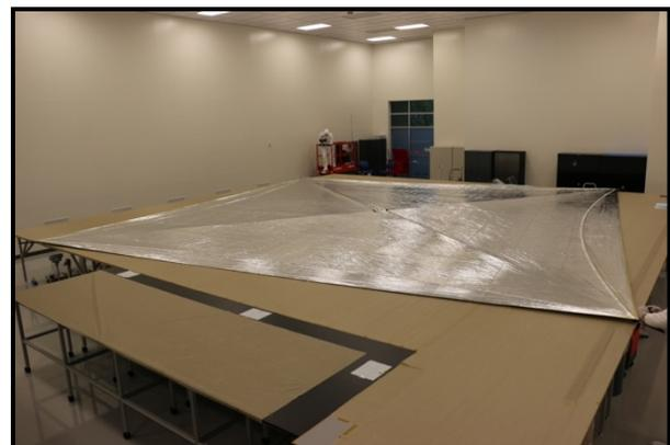
**Figure 13: Solar Sail Subsystem Flight Unit, Deployed**
