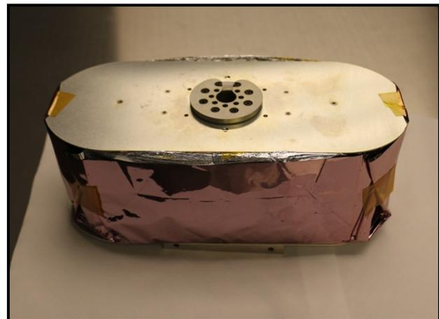
**Figure 12: Solar Sail Flight Unit, spooled**
