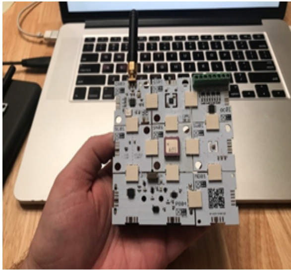
Fig. 3. A FlatSat created by students in the Remote Sensing course.
