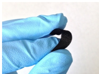
Figure 3. A digital photograph showing the flexibility of the PEDOT(IL)-coated carbon cloth.
