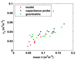
FIG. 8. Spatial std dev of 800-m, 30-min gridded modeled (red), in situ capacitance probe (black), and gravimetric (green) soil moisture as a function of spatially averaged soil moisture for the 11 days during which gravimetric sampling was done during SMEX04.
