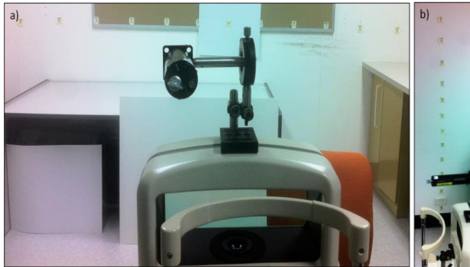
Figure 3:5: Shin-Nippon SRW 5000 auto-refractor setup for measuring central and peripheral refraction. Target placement for a) horizontal and b) vertical visual fields. An external attachment with laser light was fixed to the top of the instrument to show targets to myopic participants.
