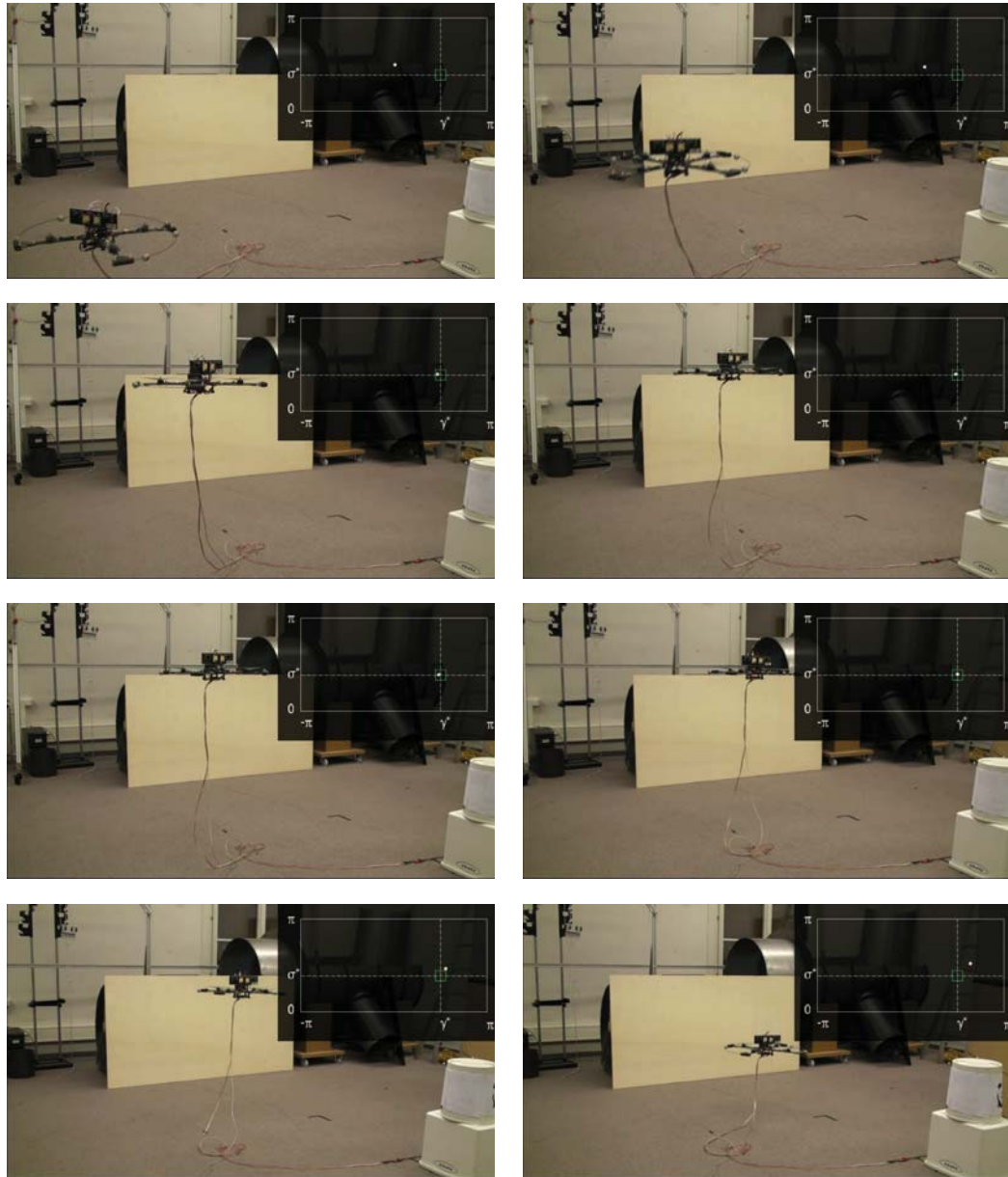
Figure 5.19: Example flight trial using spherical visual predictive control for collision avoidance of a virtual object positioned at the white cylinder. The controller regulates the image feature motion ( insert ) to the reference position \mathbf{s}^*(80\pi/180, \pi/2) ( \square ), avoiding the object by spiralling to the left. The image features then diverges ( \circ ) as the quadrotor returns to its initial altitude and heading. The tether provides power to the platform and restricts motion in the confined environment. The encounter evolves from t = 0 s ( upper left ) to t < 20 s ( lower right )
