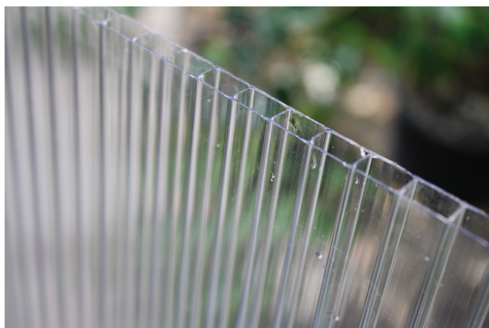
Figure 3. Twin wall ( left ) and corrugated polycarbonate panels ( right ) provide options for walls.
