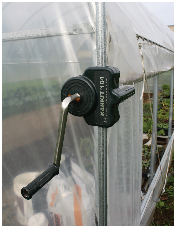
Figure 6. Hand crank roll-up window vent machine
