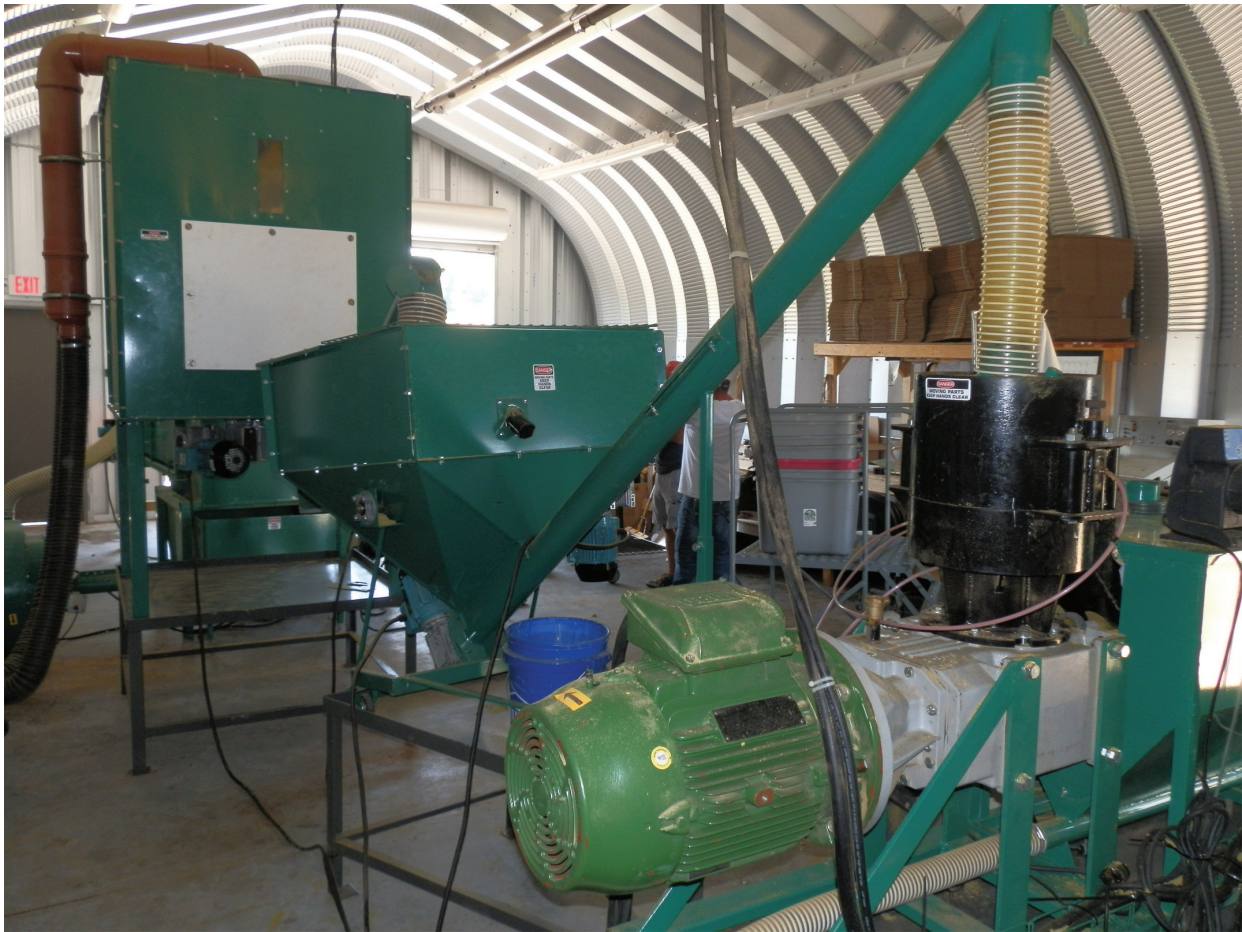
Figure 3. Hop cone pellet processing line includes a cone sieve, hammer mill, pelletizer, and pellet sieve. It is important to note that pellets are considered a food product and may require strict food processing guidelines and specialized equipment.
