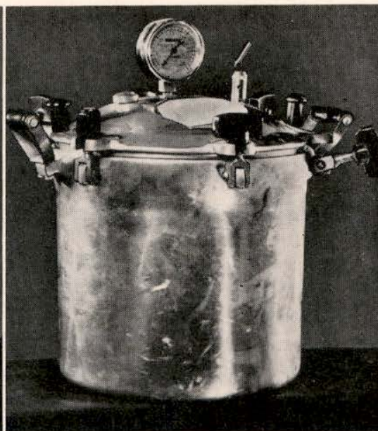
FIG. 2.—Cooker II, twelve-quart aluminum conventional-type seal using yoke bolts and wing nuts. Satisfactory dial on pressure gauge. Safety valve and petcock combined. Small knob at left of pressure gauge is a safety plug.
