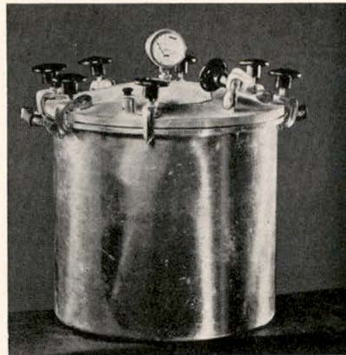
FIG. 3.—Cooker III, eighteen-quart aluminum, bead-and-groove-type seal using "C" clamps. Pressure gauge dial unsatisfactory because pointer movement is too small. Combined safety valve and petcock not the best because petcock must be held open to release air and steam.
