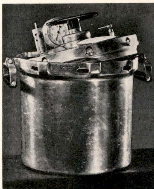
FIG. 1.—Cooker I, eleven-quart aluminum with central sealing device. Satisfactory dial on pressure gauge. The petcock was improved in the laboratory by adding a small bar which made closing and opening easier.
