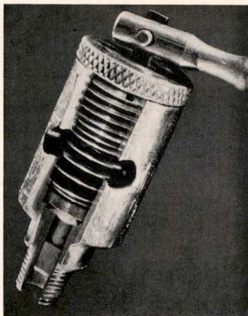
FIG. 11.—Modified needle valve, also a combined safety valve and petcock. This is satisfactory but has the drawback that the valve seat is hard to clean.
