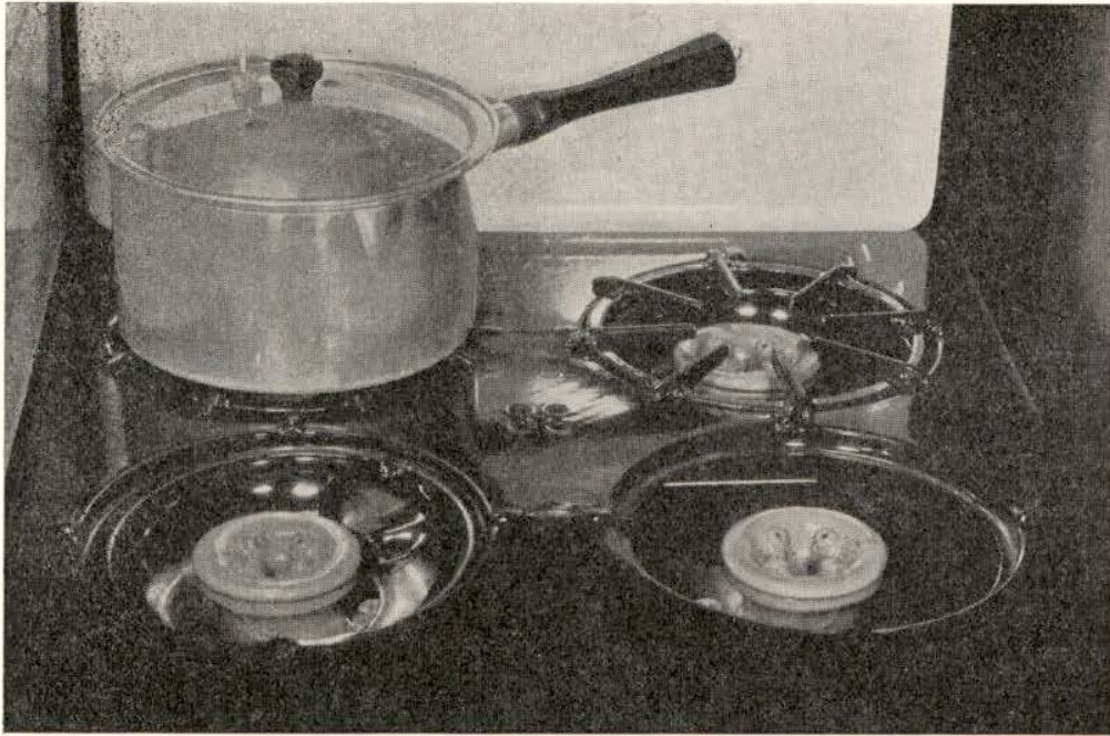
FIG. 8.—Enclosed top with round ribbon-flame burner. The burner is \frac{7}{8} inches from the top of the grate. The flame burns horizontally from the side of the burner. The utensil is a three-quart aluminum sauce pan, bottom diameter 7 inches.
