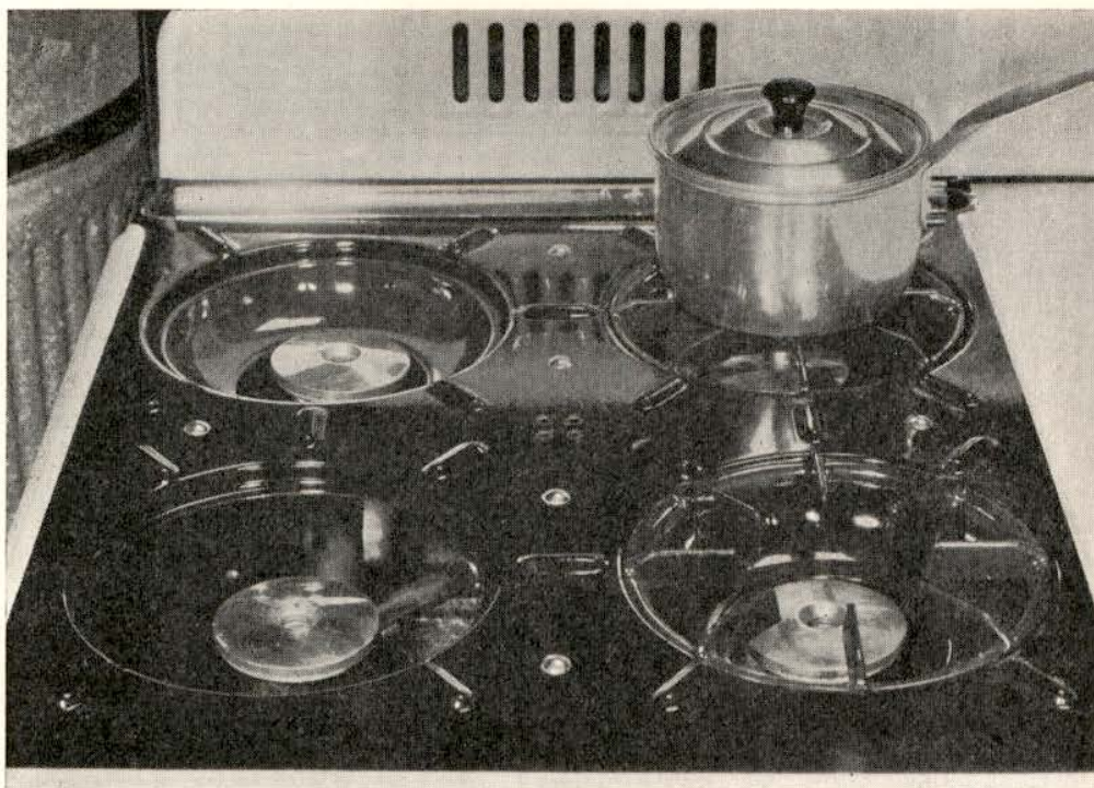
FIG. 4.—Enclosed cooking top with die-cast burners and removable burner bowls. The burner is adjustable in height, the shortest distance to the top of the grate being 1\frac{3}{8} inches. The flame is the ribbon type, burning horizontally. The utensil is a one-quart aluminum sauce pan, bottom diameter 4\frac{3}{8} inches.
