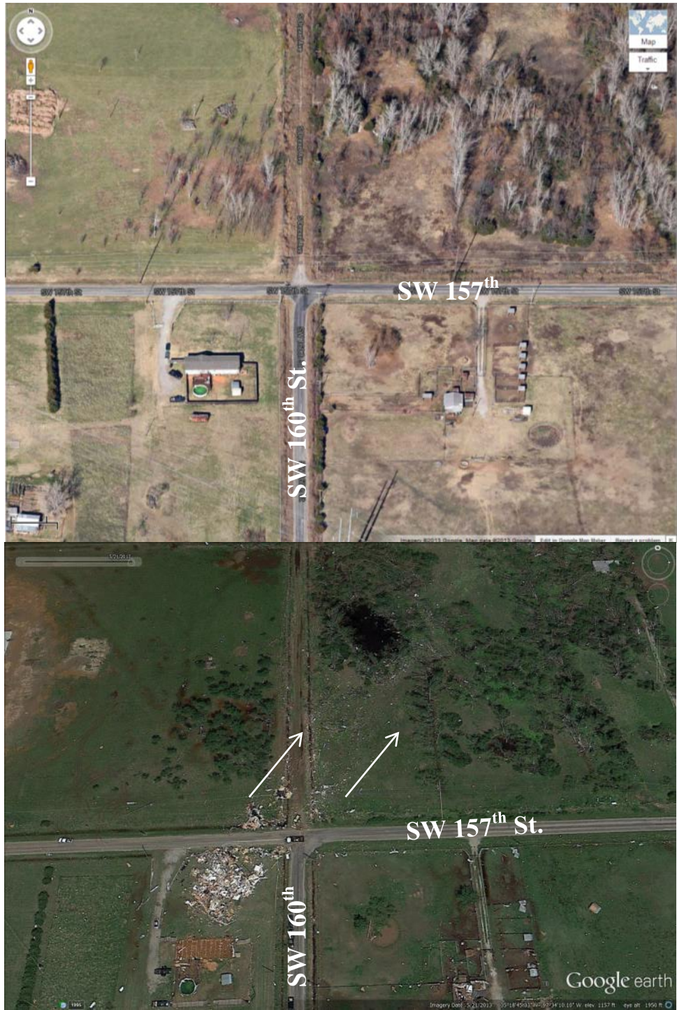
Figure 6.23, Debris Flow 2 -- Spreading in direction of tornado travel
