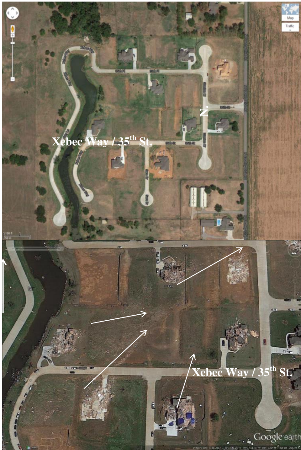
Figure 6.22, Debris Flow 1 -- Approximately Parallel to Tornado Path
