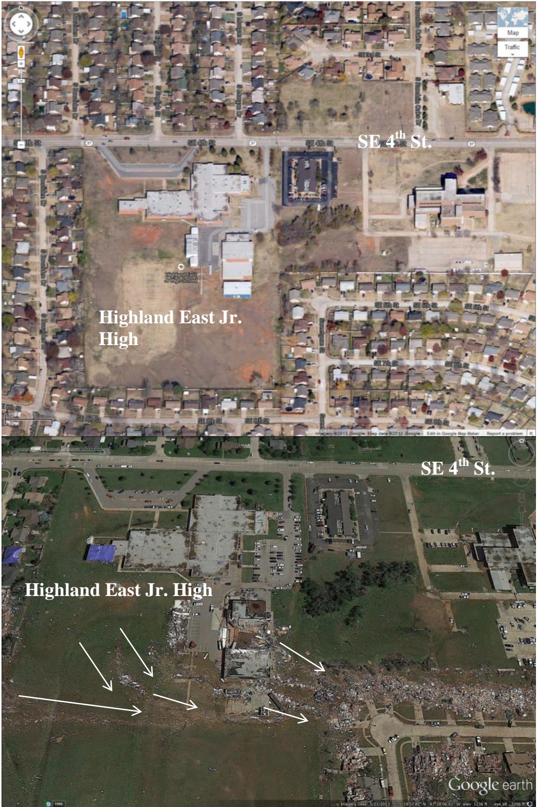
Figure 6.25, Debris Flow 4 – Debris Lines from Highland East
