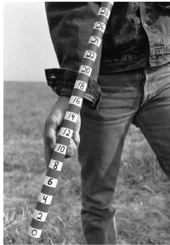
Figure 2. A modified Robel pole with 2-cm bands was used to measure the height and density of residual cover at sharp-tailed grouse nests and along landscape-scale transects on the Bessey Ranger District, Nebraska National Forest, Nebraska, USA, 1988–1990. If all or some of the bottom band was visible, the visual obstruction reading was recorded as zero indicating the number of bands totally obscured from view.
