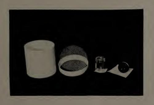
Figure II Holding cage and feeder bottle used in tests.
