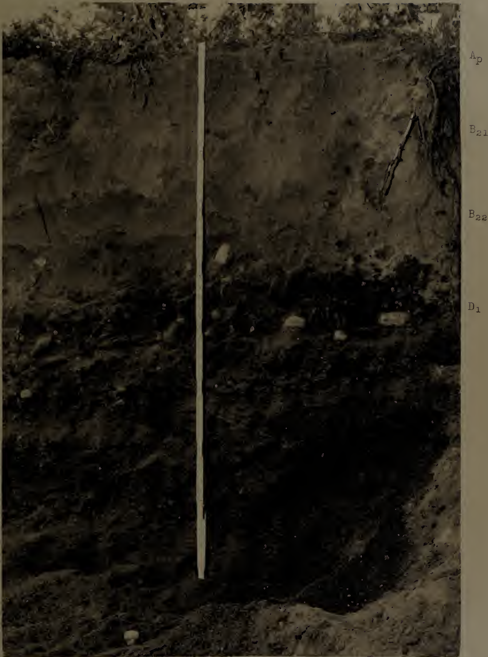
Figure 4. Close-up of Enfield silt loam (over outwash sand and gravel) in figure 1. Note the sharp contact between the underlying stratified outwash materials and the overlying profile developed in loess. An old plow layer ( A_p ) is present in the upper 6 inches of loess. The remainder (6-24 inches) of the profile constitutes the B horizon and the underlying stratified sand and gravel the D horizon. No C horizon is present in this profile. Photo taken August 6, 1953.
