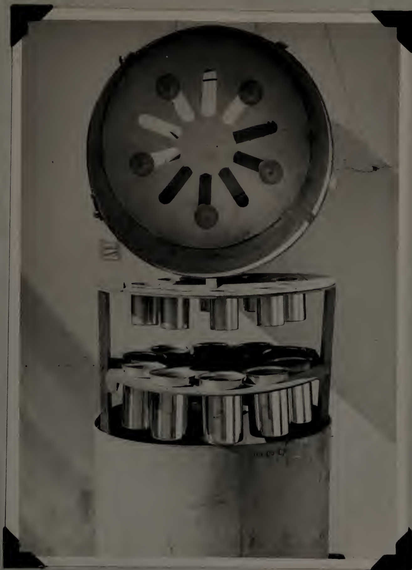
Figure 1. Breakdown view showing use of calorimeter cans and light source as used in moisture evaporation experiment.
