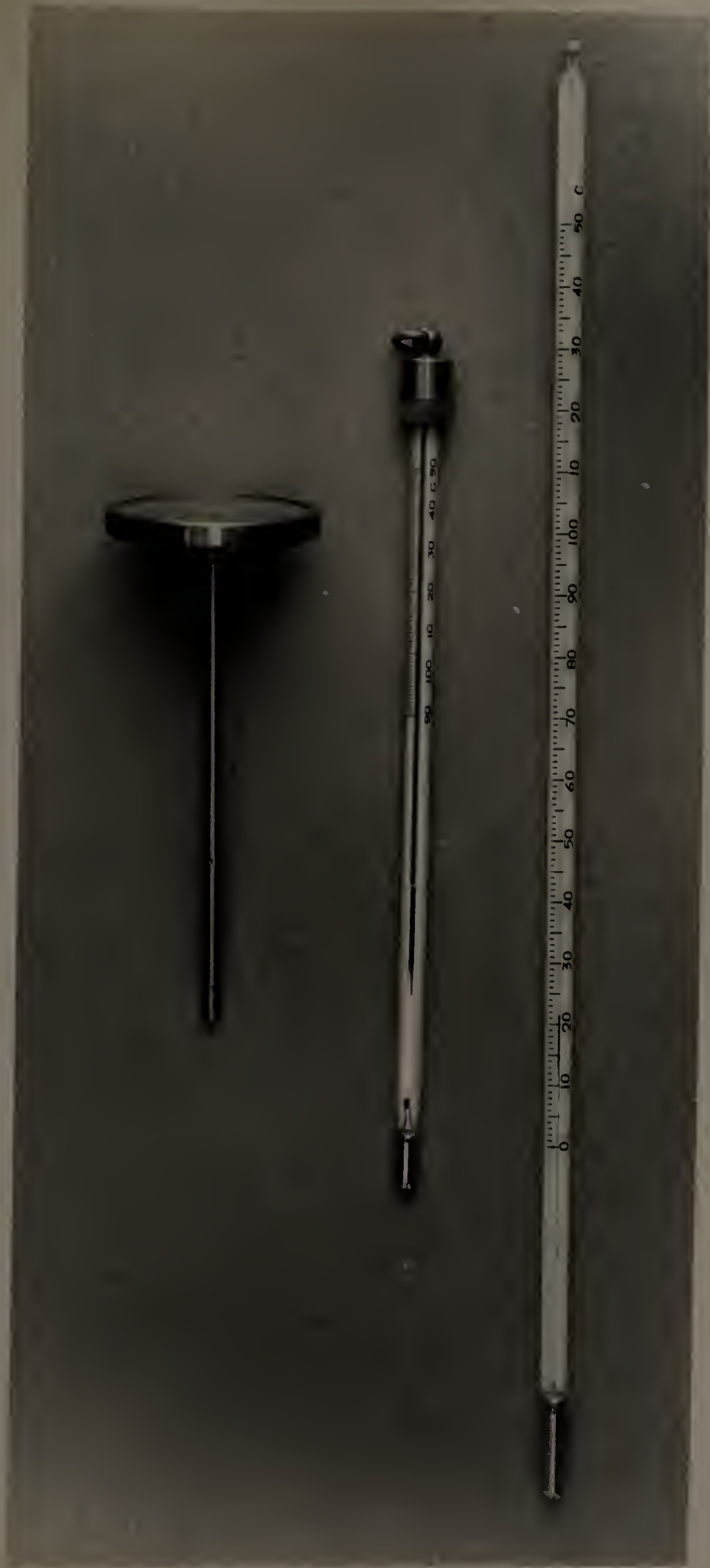
Thermometers used for measuring well temperatures in Aerovaps, from left to right: Weston bayonet, pocket, and laboratory.
