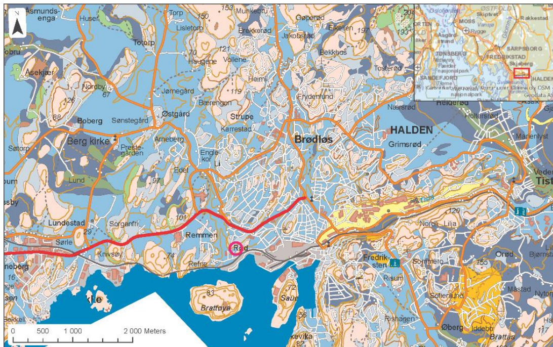
Figure 2.3 Quaternary map of the Halden area, Southeast Norway, with the research site circled in red. The colors reflect the geological processes and general properties of the deposits. Shades of blue indicate that the soils have been transported by and deposited in a marine environment. These deposits dominate the Halden area. Shades of green indicate soils that were deposited by the ice. Shades of yellow indicate fluvial deposits, and pink shows exposed bedrock. After Olsen and Sørensen (1993).
