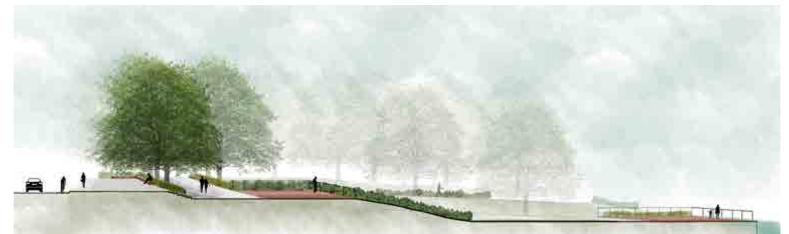
Three terraces structure Harriet Tubman Park. The first one is level with Hickory Street, the second one contains a long, central promenade and the third is a large open green space with a deck over the water.
