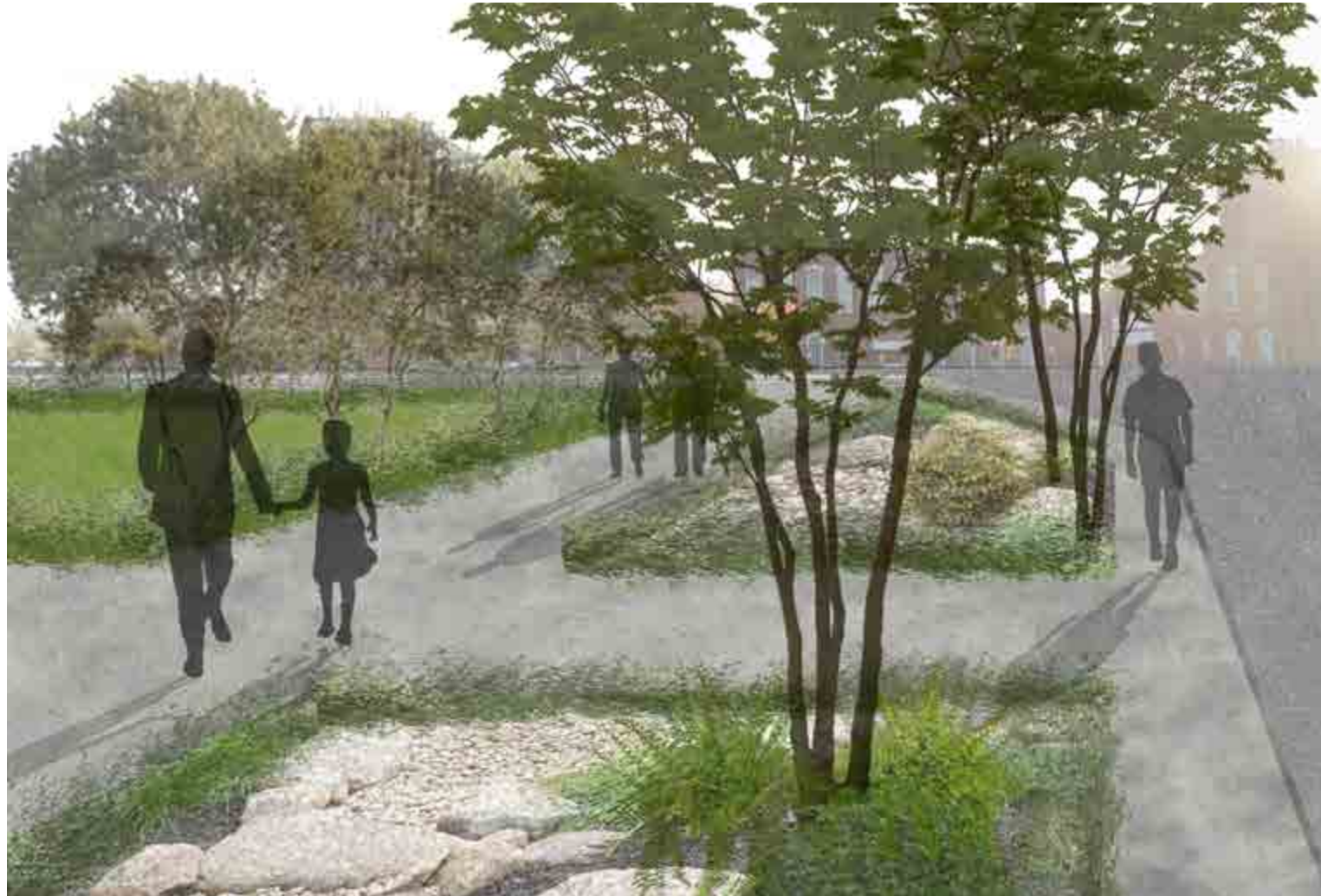
A view of the walk and vegetated edge on Rifle Street. The vegetated edge captures stormwater from Rifle Street and cleanses it before it is conveyed into the Mill River.
