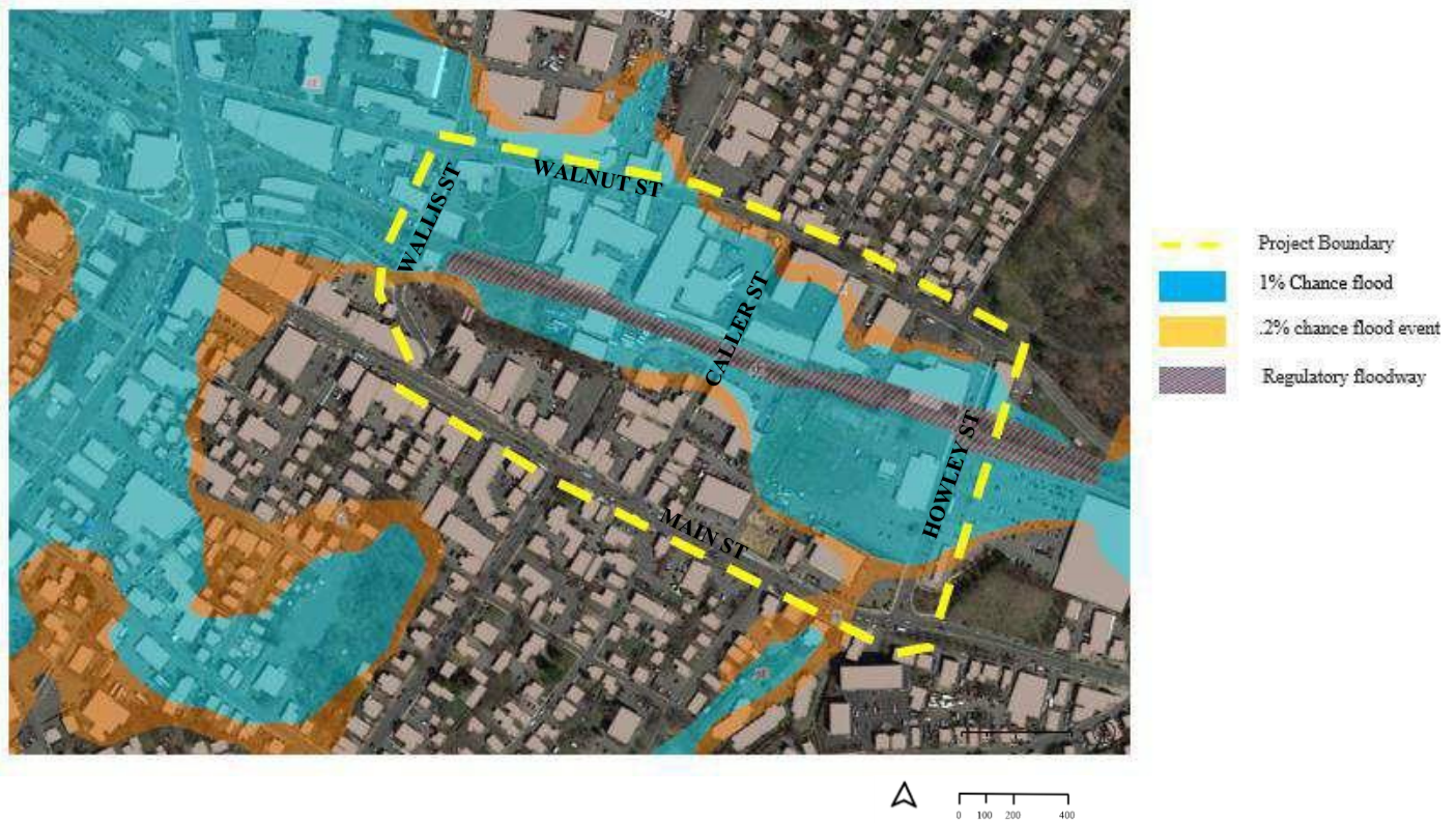
Fig. 16: FEMA flood map. The flood prone areas are indicated within the project site. (Courtesy of FEMA)
