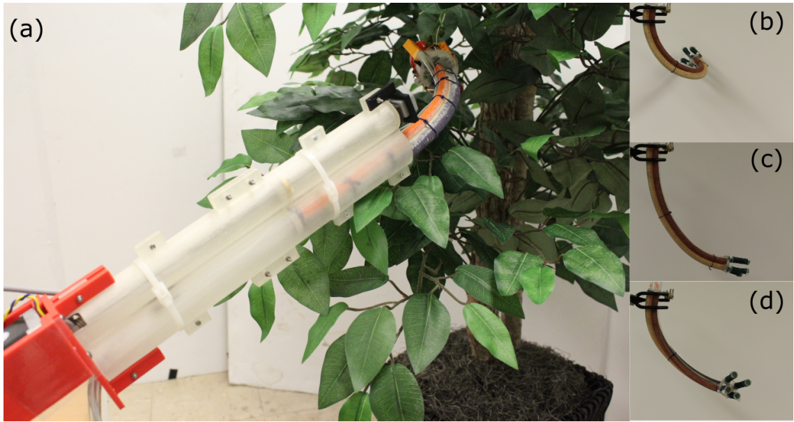
Figure 2.2: (a)Gripping an artificial tomato in an occluded environment using a VaLeNS arm with extended soft manipulator (b-c) A BR2 manipulator showing the range of motion achievable.
