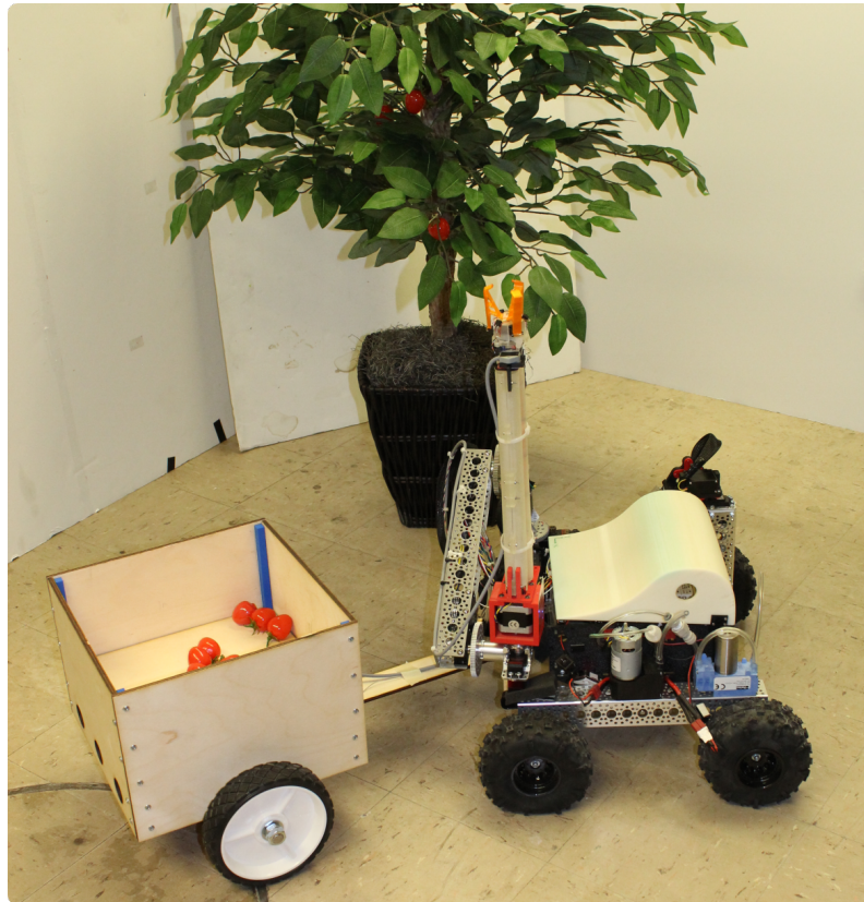
Figure 2.1: SoftAgbot - A mobile berry picking system that uses a hybrid soft-rigid arm to safely reach inside a plant and pick fruit
