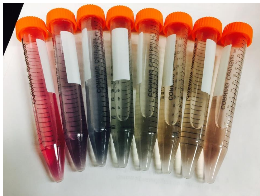
Figure 1.2. (a) A UV- vis absorption spectrum for Au NPs in water with different aspect ratios. The longitudinal \lambda_{\text{max}} increases with aspect ratio. (b) A picture of Au NP solution with an increased aspect ratio from left to right.
